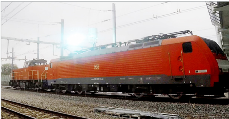
Figure 5: Reaching the short-circuit zone while passing through the system separation section with voltage detection deactivated (Photo: ProRail).
