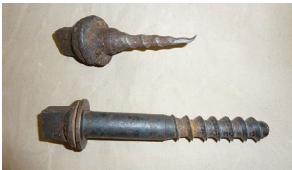
Corrosion damage due to stray currents, at a sleeper screw. Top affected, bottom new © Ulrich Bette, Institut für Beeinflussungsfragen Wuppertal
