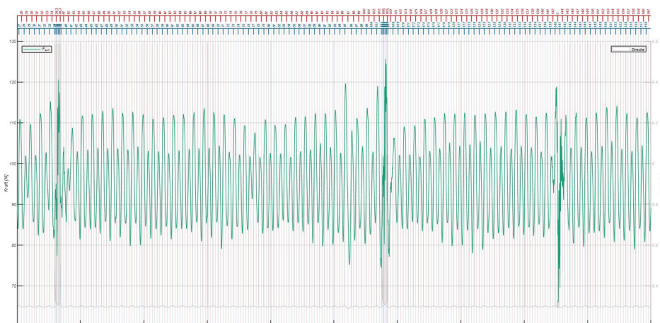
Curve of contact force with mounting condition of the overhead contact line conductor rail
